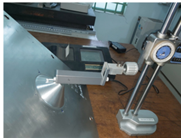
Fig. 8. Measuring outer surface roughness of a frustum cone product by surface roughness measuring machine
