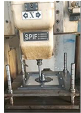
Fig. 3. Practical model of Jig and fixture system for TPIF process
