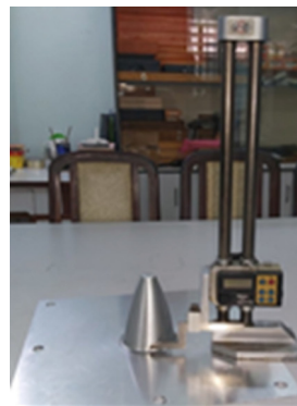
Fig. 6. Measuring the forming height
