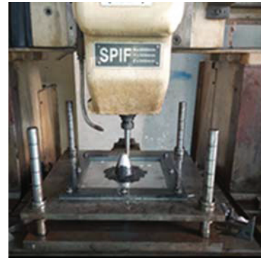
Fig.2 Practical model of Jig and TPIF process.
